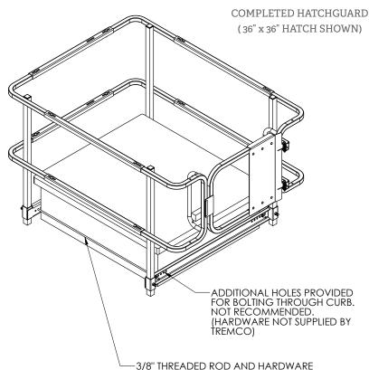
3/8" THREADED ROD AND HARDWARE FOR COMPRESSION MOUNTING
