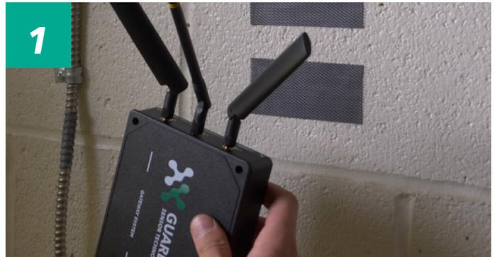
2. PLACE THE SMARTGATEWAY ON A SHELF OR USE INDUSTRIAL VELCRO TO MOUNT ON THE WALL. PLUG THE POWER ADAPTER INTO THE ELECTRICAL OUTLET.
